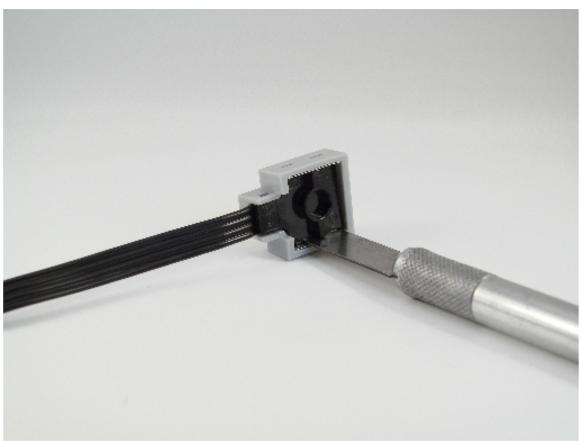
Using a small flat tool, pry both sides of the gray housing away from the black insert.
