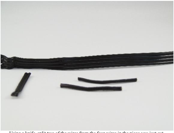
Using a knife, split two of the wires from the four wires in the piece you just cut.
