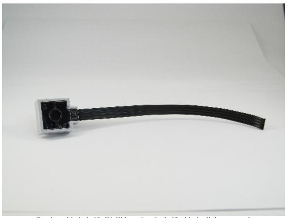
Cut the cable in half. We'll be using the half with the light gray end.
