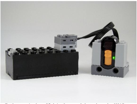
Test by connecting the modified piece between a 9v battery box and an 8884 Power Functions IR Receiver and powering the unit up. Green light = good. No light = bad.
