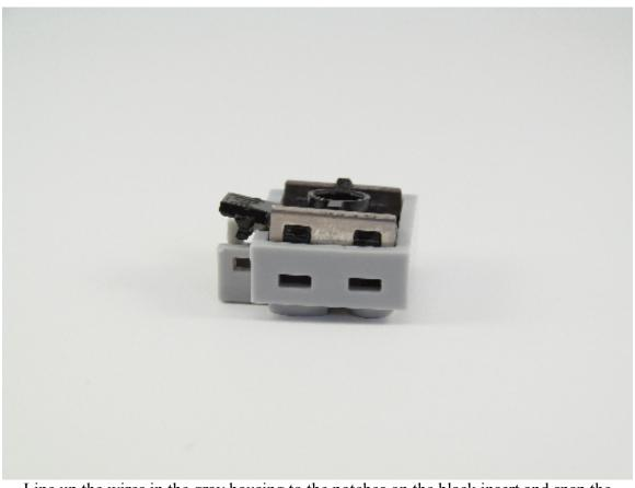
Line up the wires in the gray housing to the notches on the black insert and snap the insert back into place.
