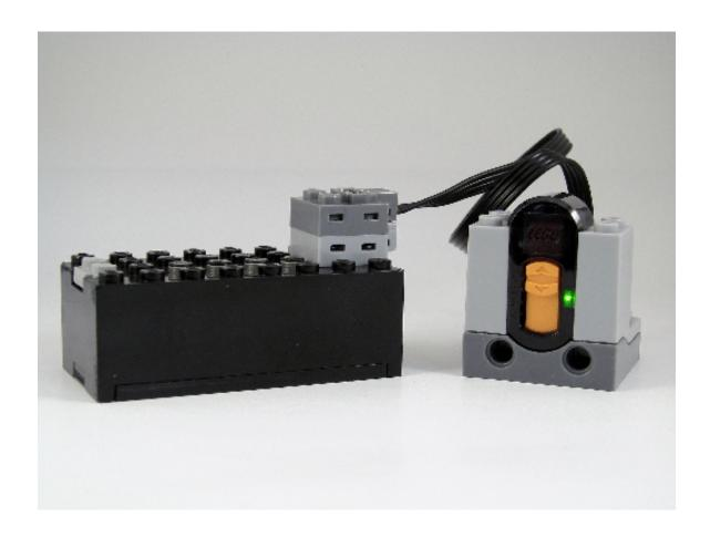
This tutorial will show you how to modify an 8886 Power Functions Extension Wire to allow you to use your 8884 Power Functions IR Receiver with the now "older" style 9v battery box, the 9v train speed regulator, RCX, etc. This could come in very handy in some space-constrained models (1x9v battery box) or in places where mains power was more suitable (train speed regulator).
